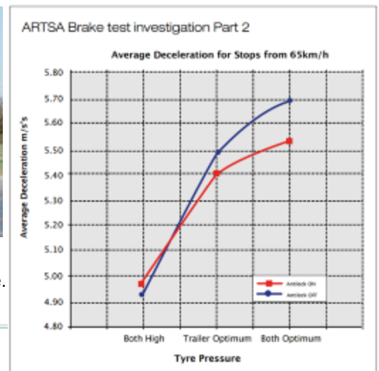
The vehicle with optimum tyre pressure achieves about a 15 % higher average deceleration than the vehicle with high tyre pressure.
