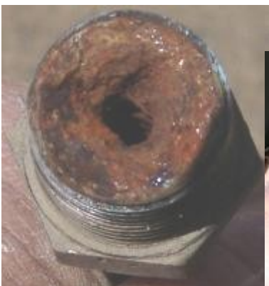
This steel armature rusted closed.
