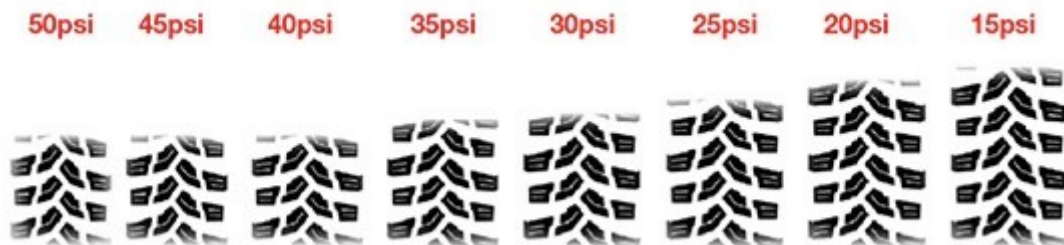
Footprint increases as tyre pressure reduces (SUV shown).
