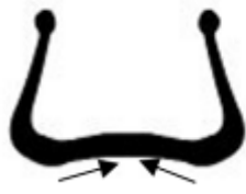
Soil pushed back inwards under low inflated
