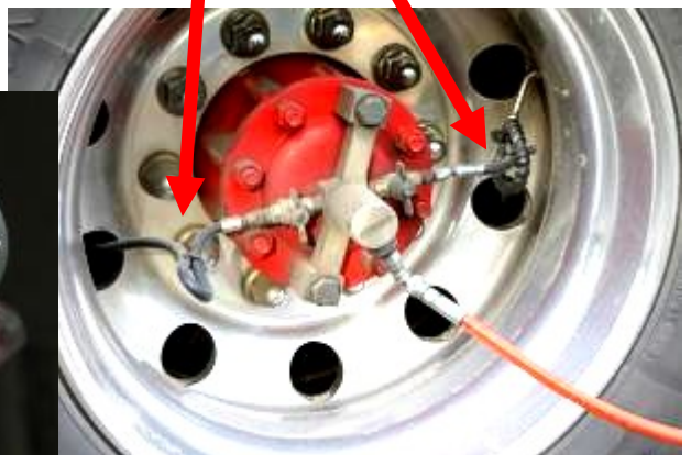
These tyre hoses were zip tied to keep from rubbing
